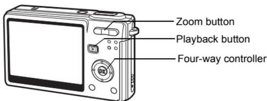
**1 Press the
