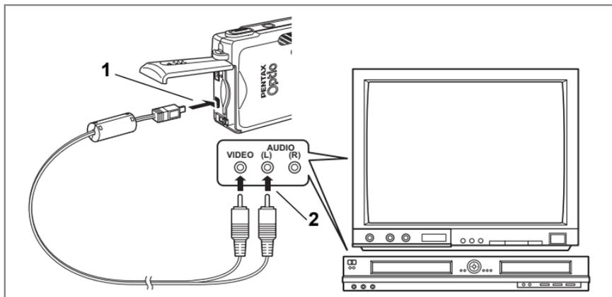
By using the AV cable, you can capture, play back and dub images on a TV or other equipment with a video IN jack. Make sure that both the AV equipment and the camera are turned off before connecting the cable.
