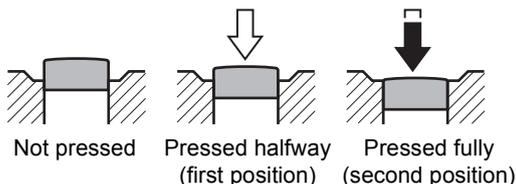
Pressing it down halfway (first position) turns on the viewfinder and LCD panel indicators and the autofocus system operates. Pressing it fully (second position) takes the picture.
