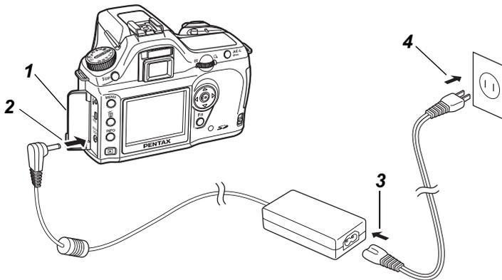
We recommend using the AC adapter D-AC10 (optional) when using the LCD monitor for a long time or when connecting to your PC.
